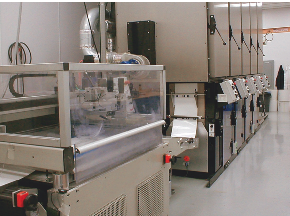
GSI prints RFID antennas on a 20-in., flatbed, single-pass, web conductive printing line equipped with 96 ft of drying capacity.
