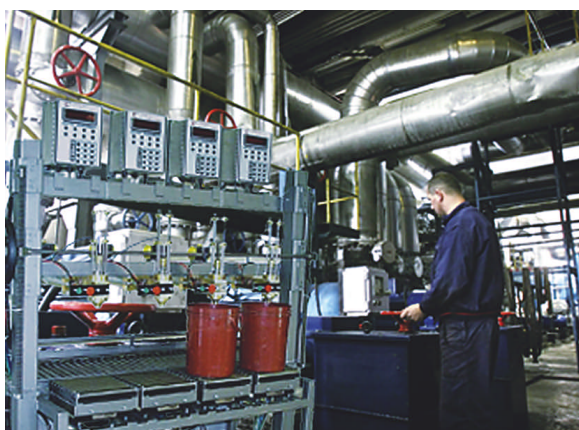
Fillers, above, shipped to third-world countries can experience problems caused by bad power supplies. Uninterruptible power systems, top photo, eliminate these problems by creating clean power on a continuous basis.
